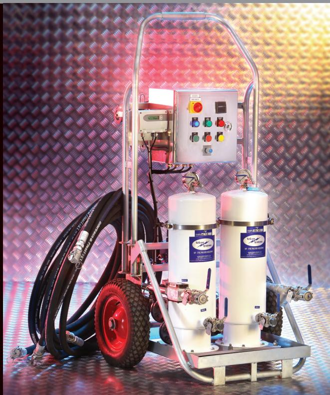
The dual housing filtration trolley, Model OF2-1000, is designed for the removal of particulate and moisture from oil used in electrical plant – where a high dielectric strength and low moisture content are specified. Quality oil to specification is guaranteed at point of use.
